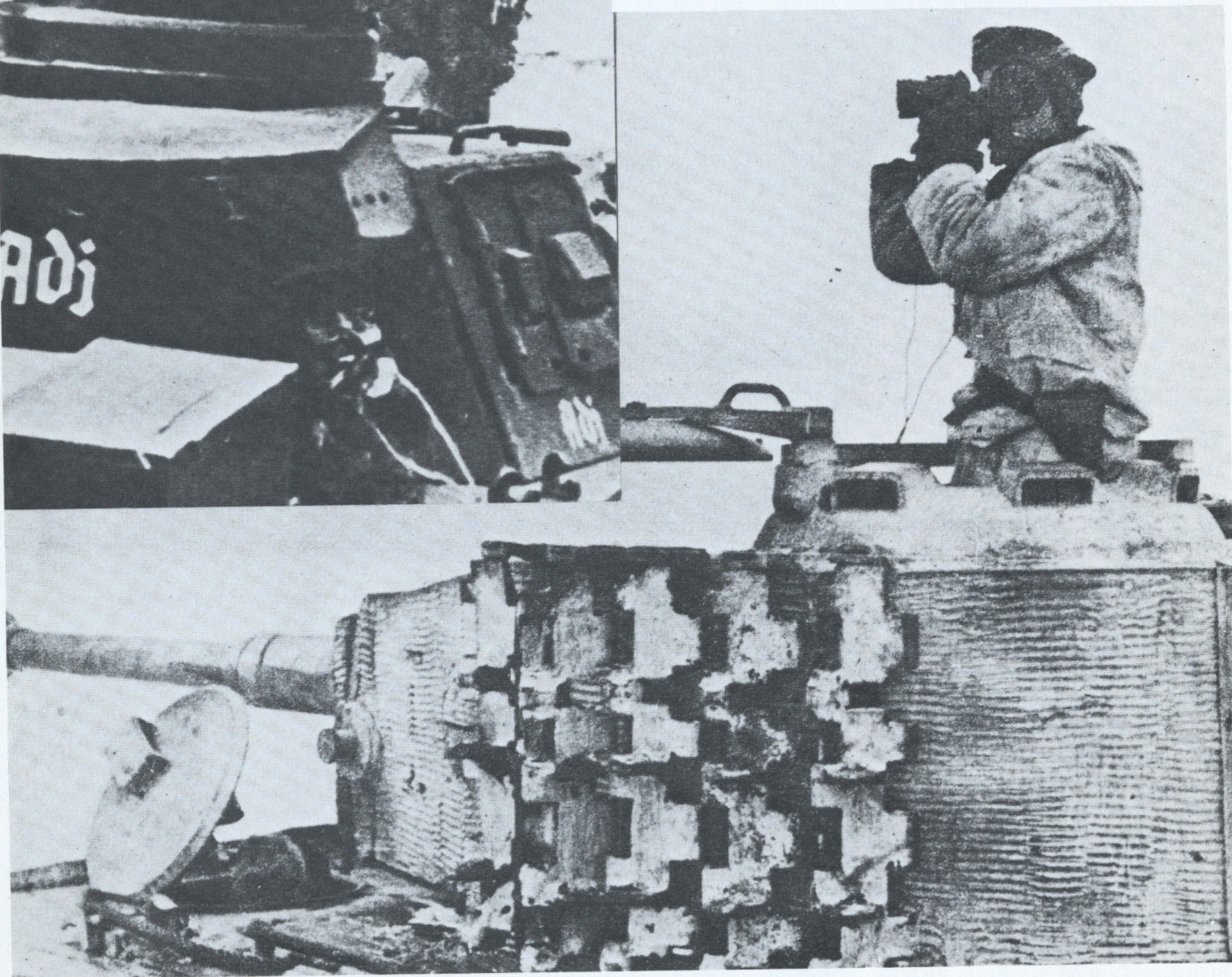
BELOW: Very neatly applied 'zimmerit' on a whitewashed battalion commanders late production Tiger.
